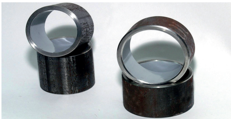
Figure 5 - Tubing with polymer coating PEP-585.
